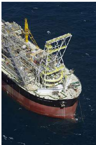
Internal Disconnectable Turret
